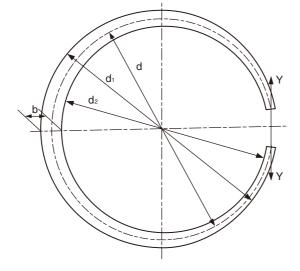
If the average curvature radius in the free condition is changed to  $\rho$  by spreading the ring in the Y directions as shown in the figure, this relationship is given by the following equation.
